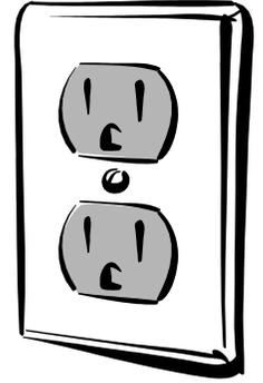
**NEC 406.9.** Receptacles not located under an overhang, canopy, or otherwise protected from the weather are to have an "in-use" , a.k.a "box hood" cover installed to protect the cord connection. *The cover is to be listed for "extra duty" use.* Receptacles are not to be installed within the space occupied by a tub or shower.
